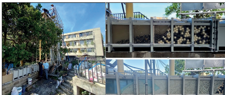
Fig. 4. Filter conformation tests at the hydraulics laboratory of NUC. Left, general perspective; Upper right, failed sand and gravel test; Lower right, successful recycled plastic filter formation. Credit: National University of Colombia.
