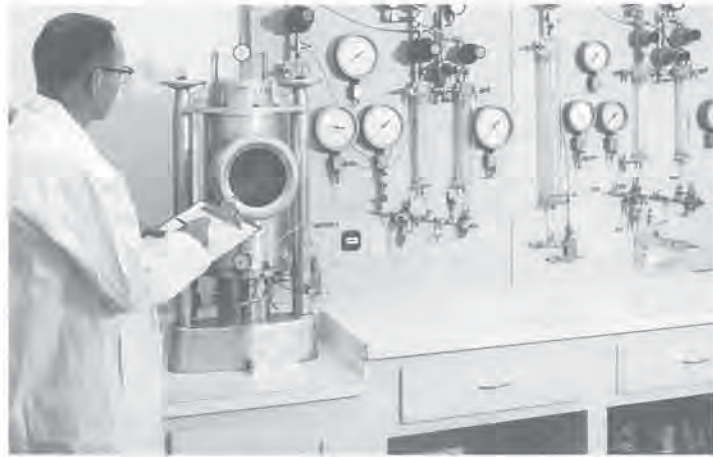
High-pressure triaxial machine. Photo: Mathieson Photo Service
