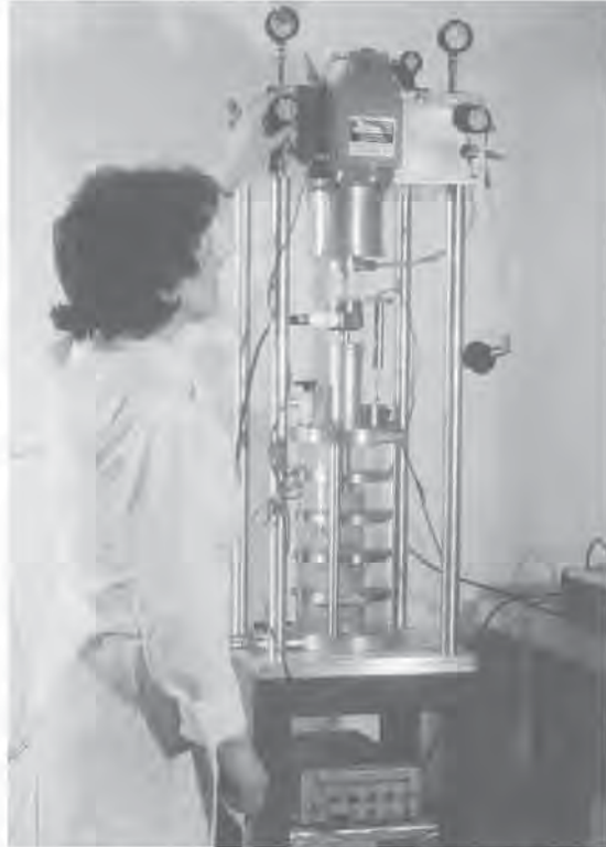
Jenny MacDougall conducting cyclic triaxial laboratory test, Richmond, B.C., 1981.
