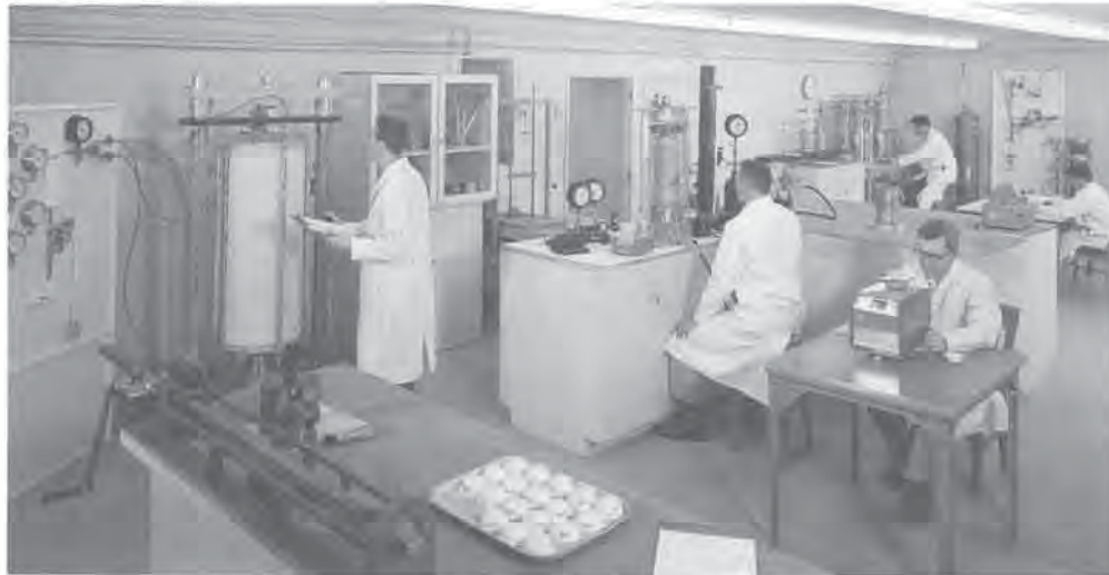
General testing room, 18-inch-diameter triaxial machine at left.
