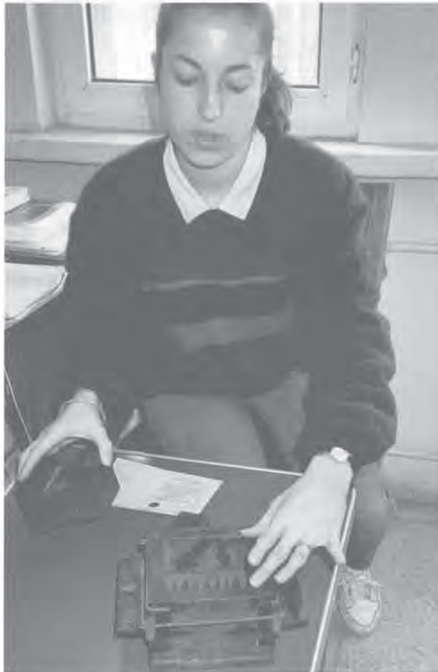
Graduate student Aysen Lav demonstrates Terzaghi’s direct shear box of 1921, Technical University of Istanbul, Turkey, October 21, 1991.
