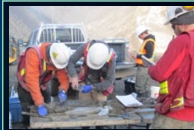
Geo-forensic fieldwork took six months and included over 1,000 soil index property tests
